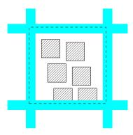
Basic DOE structure. The structure consists of 5 layers. Top and bottom are ground planes. Three layers consist of parallel interconnects orthogonal to others across each layer. The structure enables observation of intra-layer, first and second neighboring layer couplings in one simulation.
