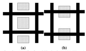
Fig. 4. Inter-layer coupling for neighboring layers. (a) Fills on layer M intersect minimally with interconnects on layers M-1 and M+1. (b) Fills on layer M shifted and intersect maximally with interconnects on layers M-1 and
