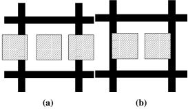
Fig. 5. Inter-layer coupling for neighboring layers. (a) Fills on layer M+1 intersect maximally with fills on layer M. (b) Fills on layer M+1 shifted and intersect minimally with interconnects on layers M.
