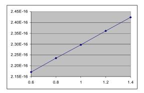
Fig. 11. CMP-induced height impact on total capacitance shows linear change.
