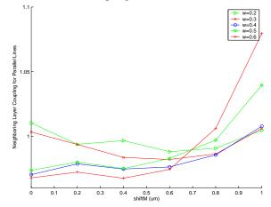
Fig. 15. Neighboring-layer parallel line coupling dependency on amount of  ${\cal M}$  layer shift for various metal widths.
