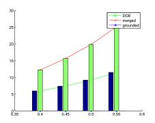
Fig. 18. Increase in coupling for DOE, merged and grounded fills for a range of metal widths.
