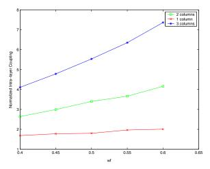
Fig. 12. Fill width dependency of intra-layer coupling for different number of fill columns.
