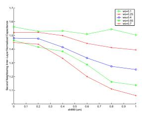
Fig. 17. Fill shift dependency of second neighboring layer coupling for different fill to fill spacings.
