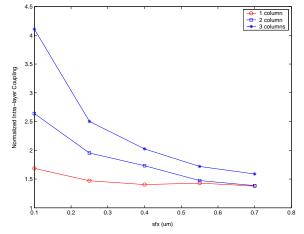
Fig. 13. Fill spacing dependency of intra-layer coupling for different number of fill columns.
