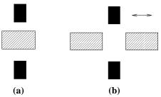
Fig. 7. **Inter-layer coupling for second neighboring layers.** (a) Fills on layer M intersect maximally with interconnects on layers M-1 and M+1. (b) Fills on layer M shifted and intersect minimally with interconnects on layers M-1 and M+1.
