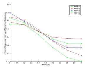
Fig. 16. Fill shift dependency of second neighboring layer coupling for different metal widths
