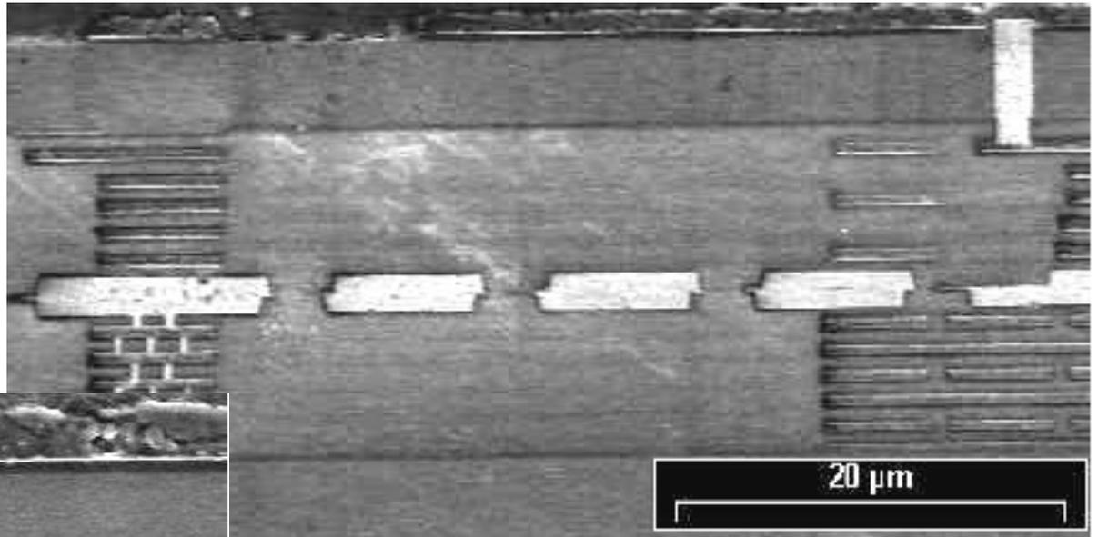
Figure 5 – SEM photo of a two-wafer stack.
