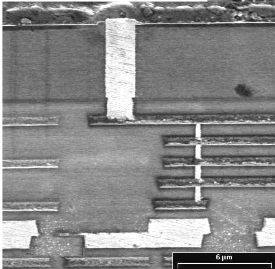
Figure 6 – SEM photo close-up of a Super-Contact.
