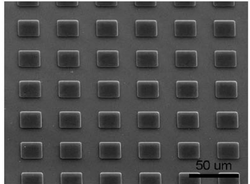
Fig. 6. SEM of an array of polysilicon islands attached to a SiO<sub>2</sub> substrate using Al-Ge eutectic bonding at 435 °C. The excess Al-Ge in between the islands has been etched away.
