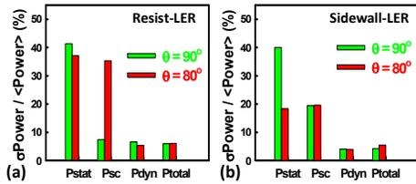
**Figure 8:** The normalized variation of each power consumption induced by (a) resist- and (b) sidewall-LER.
