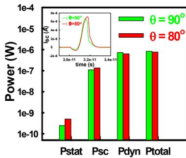
**Figure 7:** The power consumption of the nominal bulk FinFET devices and the inset is the short circuit current.
