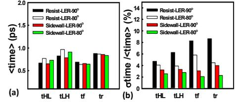
**Figure 6:** The timing of resist-/sidewall- LER on the studied bulk FinFET inverter.
