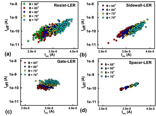
**Figure 3:** The  $I_{on}$ - $I_{off}$  characteristic of the bulk FinFETs with different fin angles under the (a) resist-LER, (b) sidewall-LER, (c) gate-LER, and (d) spacer-LER.
