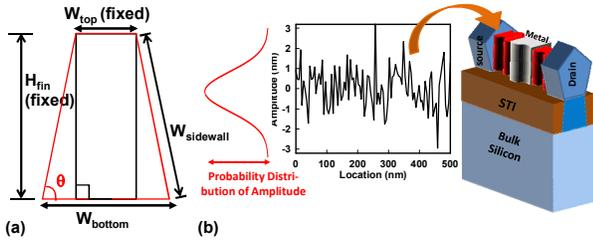
**Figure 1:** (a) Cross-sectional plot of device structure. (b) The simulation method of LER. For the LER simulation, Gaussian noise function is used to generate random edge profiles and then append them on the regular edges of nominal bulk FinFET devices. The distribution of edge amplitude follows Gaussian distribution.
