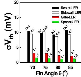
**Figure 4:** The  $V_{th}$  fluctuation of trapezoidal bulk FinFET devices with different fin angles fluctuated by LERs.
