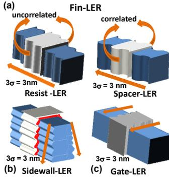
**Figure 2:** Different LER of FinFET devices. (a) Fin-LER (b) Sidewall-LER (c) Gate-LER. The fin-LER can be grouped into resist-LER and spacer-LER based on the process method. The standard deviation of each LER is set to 1 nm.
