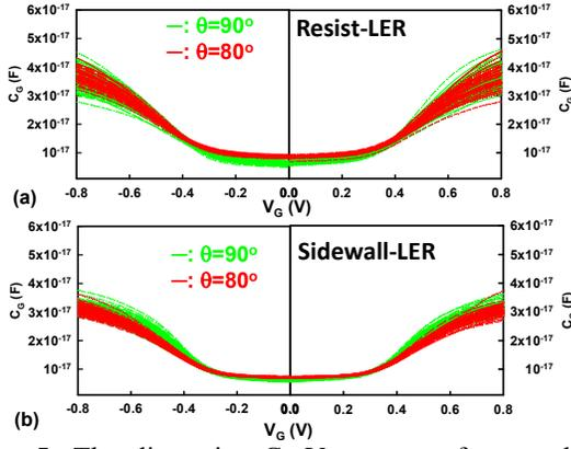
**Figure 5:** The dispersive  $C_G$ - $V_G$  curves of rectangle bulk FinFET and trapezoidal one by resist- and sidewall-LER.
