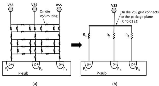
Figure 5: Illustration of the verification flow collapsing through the SRA: (a) ground grid for multiple ground path resistance into (b) a single resistance for each path from ground port to each p+ tap; the resistance at the VSS grid and package plane is negligible and ignored.
