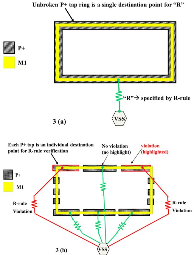
**Figure 3:** VSS NET to P+ tap ring R extraction for (a) P+ ring with continuous diffusion (b) P+ ring with broken diffusions.
