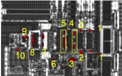
**Figure 2:** Multiple hot spots related to gate oxide damage observed at the nmos of internal nodes.
