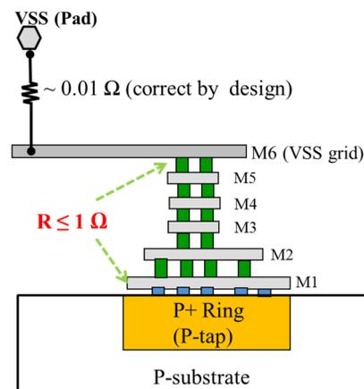
Figure 8: Allowed metal routing resistance for P+ ring to the metal\_6 (M6) VSS grid (maximum): 1 Ω
