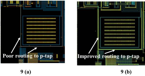
**Figure 9:** Layout snapshots for the failed and passed designs for test case (a) R-rule failed (b) R-rule passed
