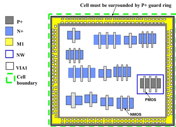
**Figure 1:** Well tap placement rule requires that the cell must be surrounded by P+ guard ring.
