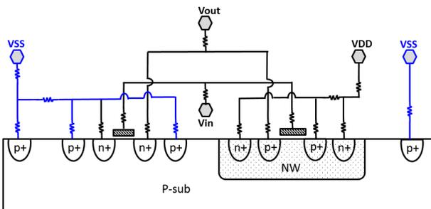
**Figure 10:** Connectivity extraction for the VSS net to the p+ well tap; the target path for extraction is highlighted in blue. Similar path selection is possible for the VDD net, or any other net of interest.
